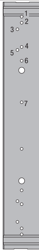
END STILE HOLE PATTERN (LEFT SIDE IS SHOWN. RIGHT SIDE IS OPPOSITE.)
